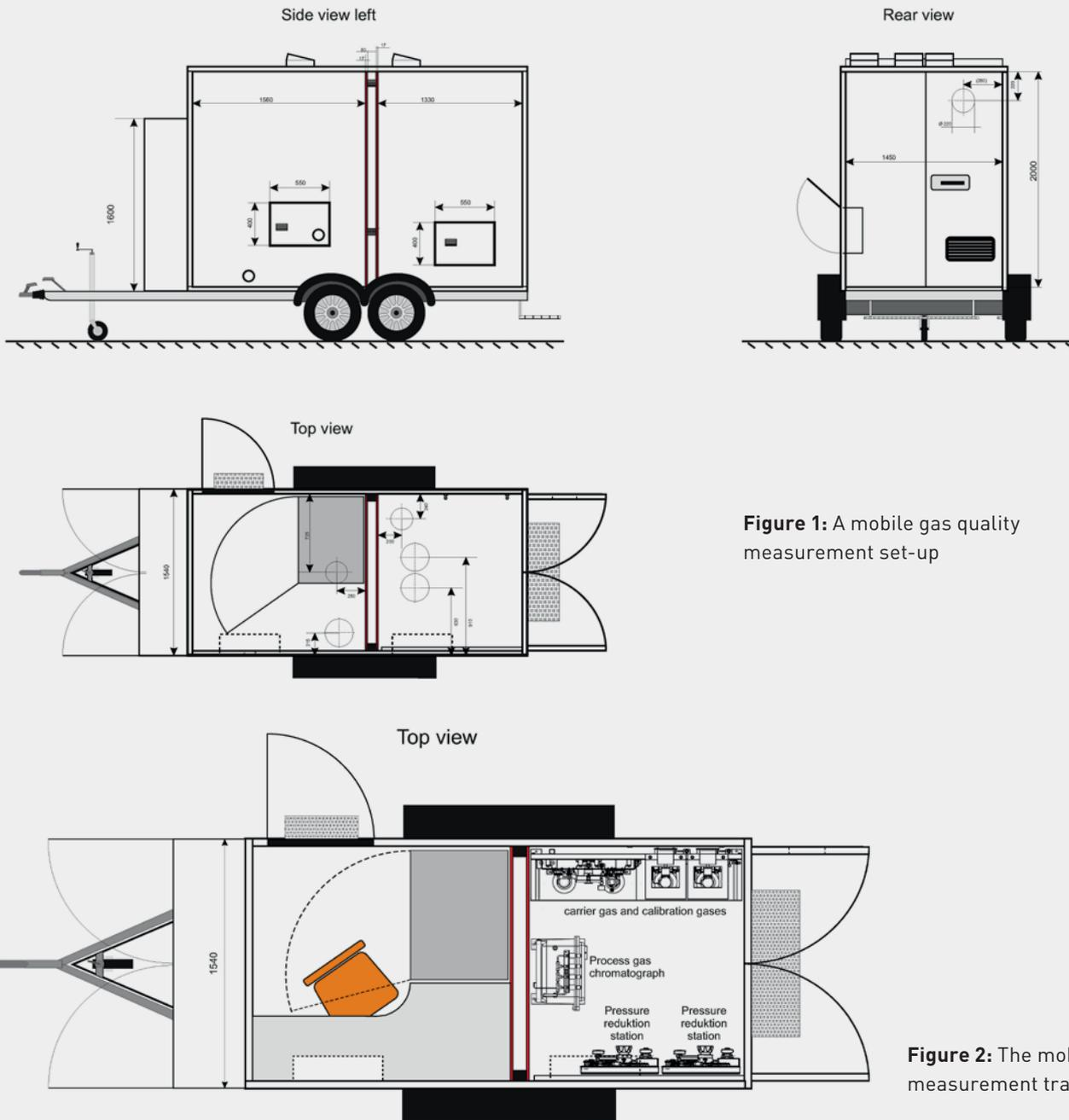
**Figure 1:** A mobile gas quality measurement set-up
