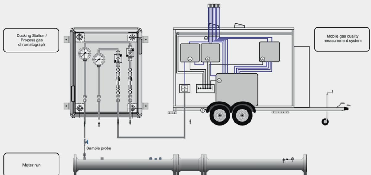
**Figure 4:** Standardized connection unit (docking station) supplies the mobile quality measurement with the natural gas to be measured
