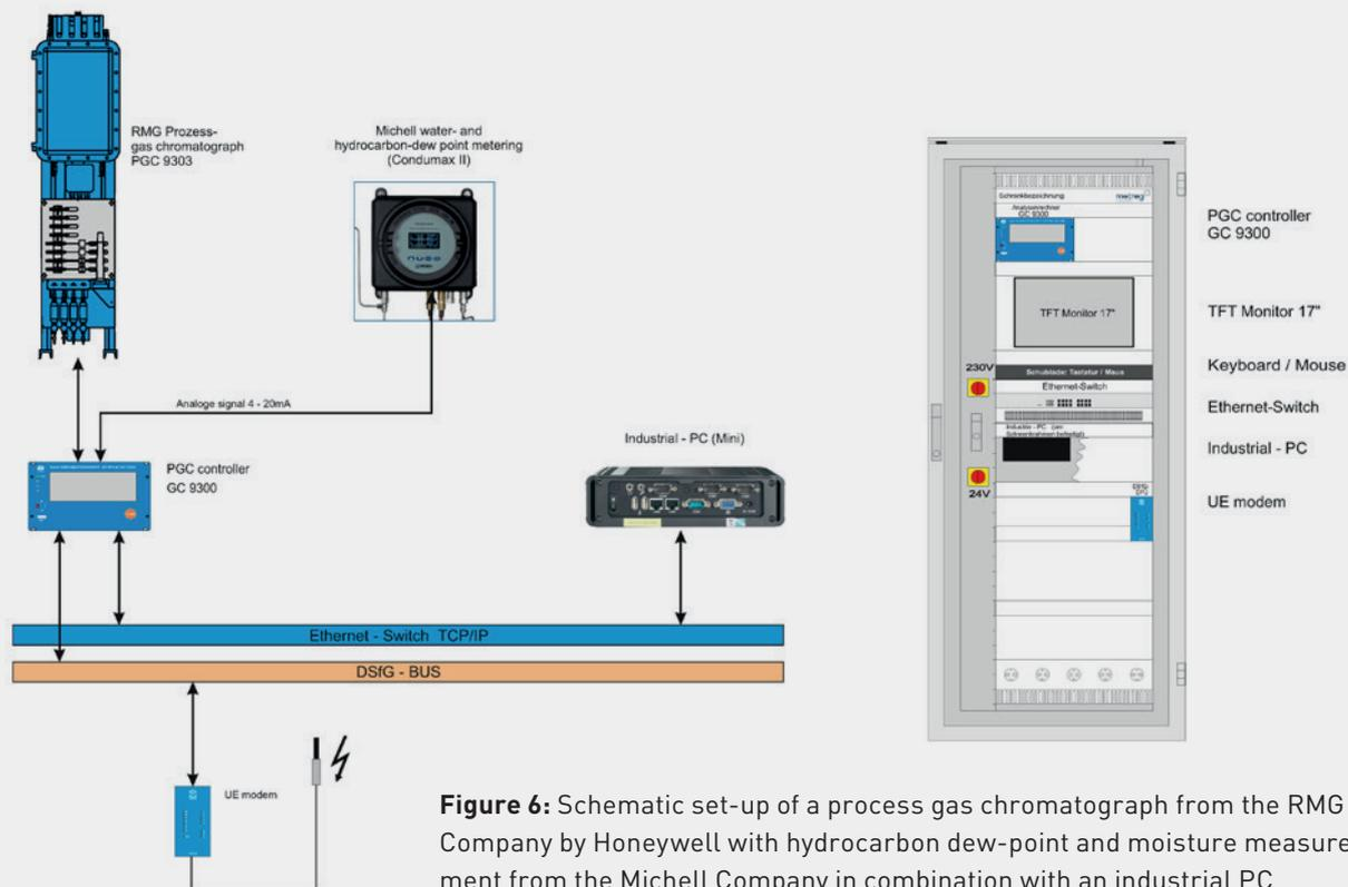
**Figure 6:** Schematic set-up of a process gas chromatograph from the RMG Company by Honeywell with hydrocarbon dew-point and moisture measurement from the Michell Company in combination with an industrial PC
