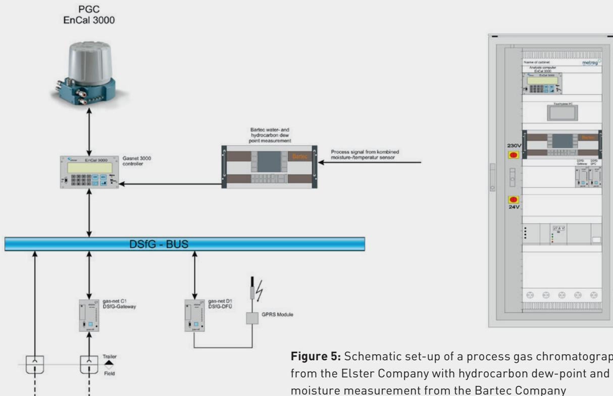
**Figure 5:** Schematic set-up of a process gas chromatograph from the Elster Company with hydrocarbon dew-point and moisture measurement from the Bartec Company
